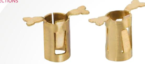
Previous designs of SMT contacts have only included 2 points of contact to the mating pin, making them potentially vulnerable to vibration. The <u>Sycamore Contact</u> patented design incorporates 3 points of contact for improved continuous signal integrity.
