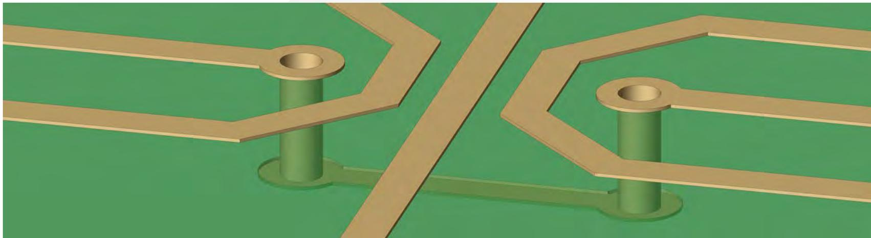
When PCB designers are laying out the PCB tracking, they may come to a point in their design where it is not possible or practical to connect all the tracks to their required origins and destinations. The current method of solving this dilemma is to break through the PCB and continue the track on the underside of the PCB, creating a second copper layer. The two ends are joined with a plated-through hole, called a via.
