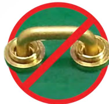
Alternative “simpler” solutions include special double-bend connectors, short lengths of wire soldered directly to the PCB, or wire jumper links in combination with sockets. These solutions all add to the component cost of the PCB, and often require a hand-soldering operation on an SMT PCB, with associated higher costs and resource requirements.
