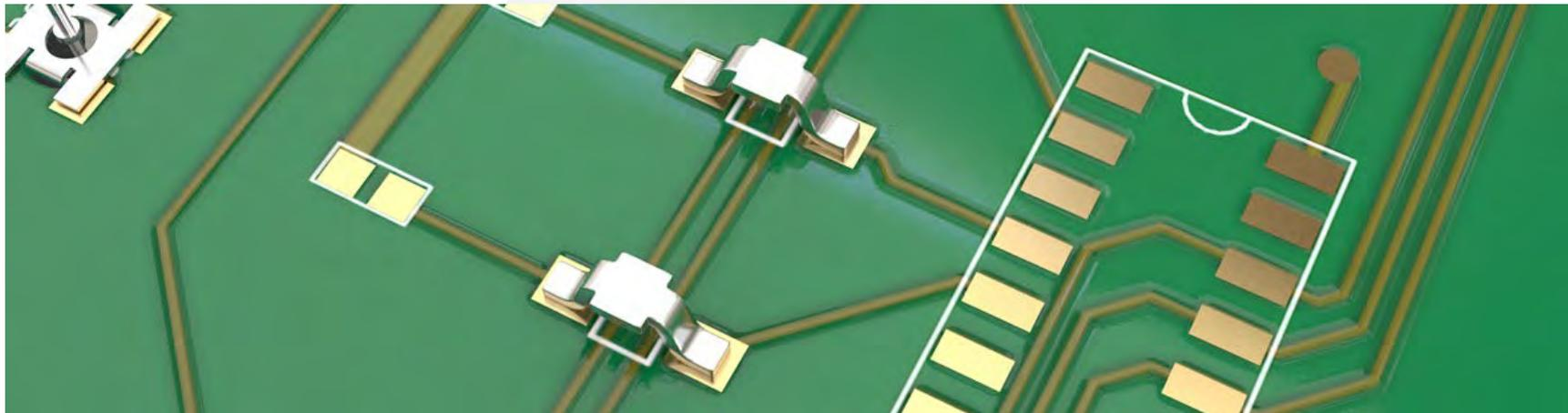
The single piece fixed SMT Jumper Links are a low-cost, easy-to-use solution for track layout problems. Acting as a physical bridge, the designer can simply jump the circuit off the PCB to reach the other side of the problematic track. Vias and double-sided PCBs can be eliminated.
