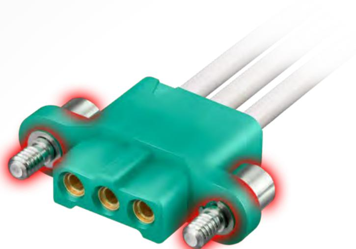
Female crimp connectors are fitted with floating Hex Socket jackscrews, suitable for 2mm Hex (Allen) keys. These will engage with jackscrews assembled in both Male Throughboard and Male Crimp connectors.
