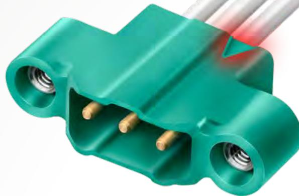
All male and female connector bodies carry a triangular-shaped inset in the housing, to indicate the position of the Number 1 contact. Counting is then continued along the row. For Double row connectors, the numbering restarts on the second row from the contact beside position 1, and continues along the row as before.
