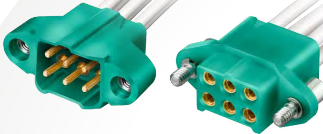
Both Male and Female cable connectors are designed to suit 18AWG to 22AWG equipment wires, with a maximum external diameter of Ø1.8mm for 18-20AWG, and Ø1.4mm max for 22AWG.
