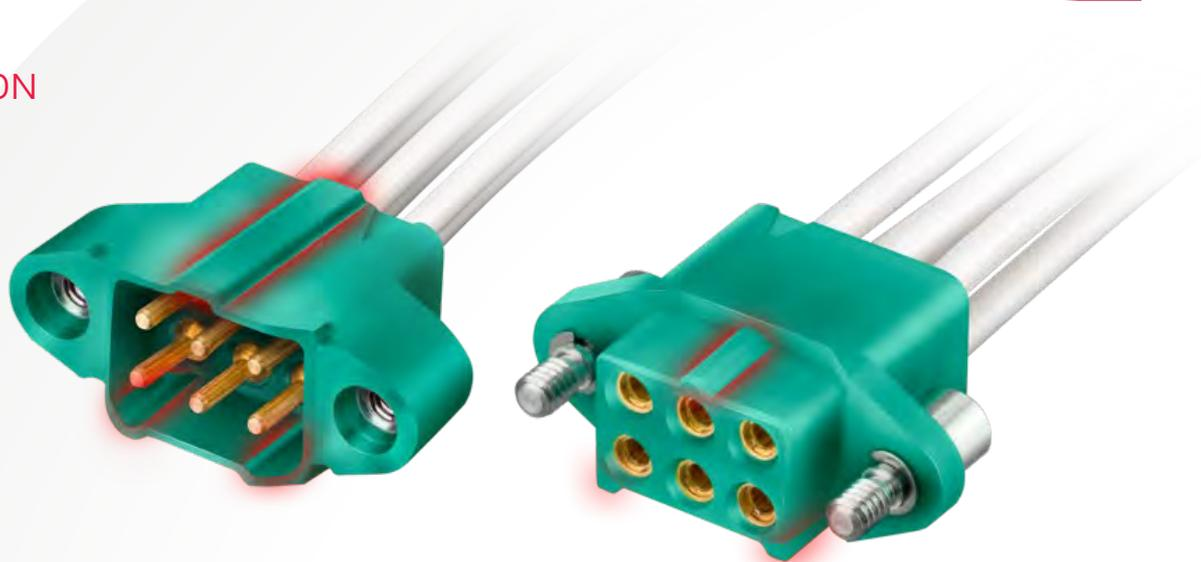
The polarization has been placed on both sides of the connector, to ensure that these connectors cannot be mated inversely. Three polarization keyways have been included in the design, on two corners and in one side.
