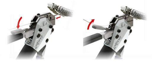
12. Position the buckle of the Microband tie behind the ridge on the backshell cable exit. Rotate the buckle to be centrally orientated on the longest side of the backshell. This is important to achieve uniform clamping of braid.
