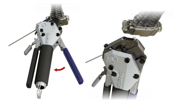
15. Remove the excess tie from the tool by pressing on the small grey handle and pull out the tail from the tool to the rear.
