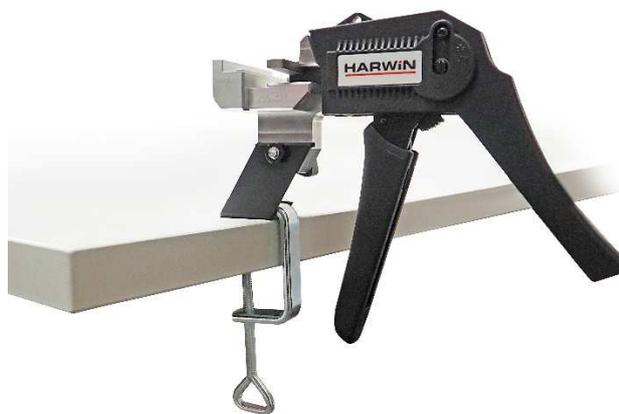
*Figure C - Tighten the clamp to the work surface*
