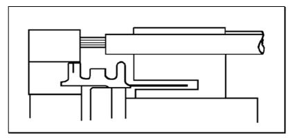
9. Hold the cable steady and fully compress the handle, to complete the crimping operation. Do not attempt to open the tool before fully compressing it, as this may damage both tool and crimp.
