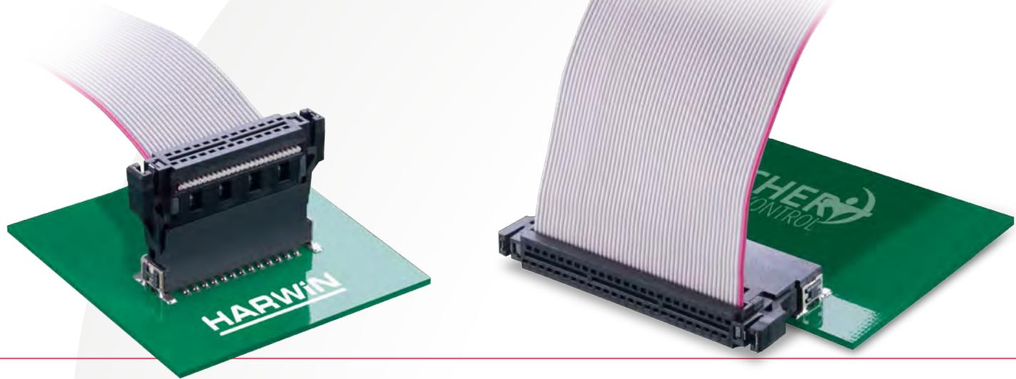
[Kontrol](#) and [Archer](#) ranges both include ready-made cable assemblies, constructed with IDC connectors and ribbon cable. The cable is UL rated with 30 AWG cores. These assemblies are available off-the shelf in 150mm, and some selections are also available from stock in 300mm. Other cable lengths can be supplied on request.
