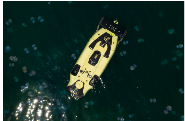
Shell's FlatFish vehicle for autonomous pipeline inspection
