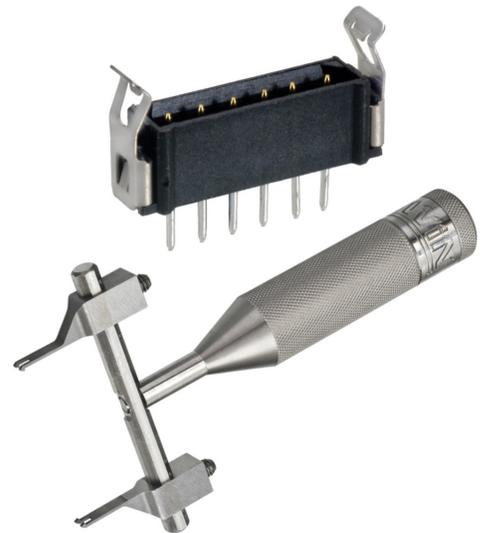
For the 1.25mm pitch Gecko series, latches were redesigned to unlatch inwards rather than outwards. This has eliminated the overstressing possibility, while still keeping real estate requirements to a minimum. These latches can be operated by hand, but tooling is also available to assist in restricted spaces. Board hold-down options are also available in both through-board and surface-mount formats.
