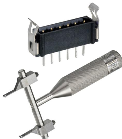
For the 1.25mm pitch Gecko series, latches were redesigned to unlatch inwards rather than outwards. This has eliminated the overstressing possibility, while still keeping real estate requirements to a minimum. These latches can be operated by hand, but tooling is also available to assist in restricted spaces. Board hold-down options are also available in both through-board and surface-mount formats.
