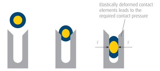
When you push the ribbon cable onto the rows of contacts, the sharp points pierce through the insulating rubber material, pushing it out the way (displacing it). As you push the cable further down, the sides of the center conductor are now in contact with the inside faces of the U channel. The conductor is squeezed slightly, ensuring a good connection joint between the cable and the contact.
