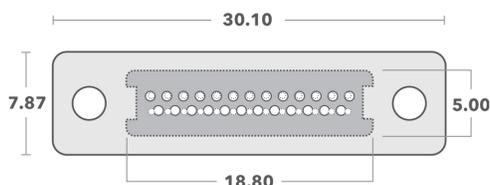
A board-to-board application will be able to use Gecko's low-profile latching system, delivering more capability than a Micro-D solution. To demonstrate this, it is possible to compare the power density delivered by each connector type. In this example, a 26-pole Gecko connector (in grey) can deliver 52 Amps (26 contacts rated at 2 Amps per contact) in a length of 18.80mm (0.740"). This leads to a power density of nearly 70.3 Amps per inch (25.4mm).
