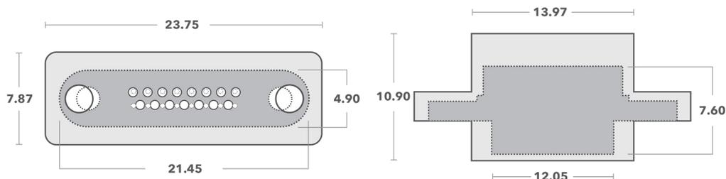
In this example, the footprint of a 16-pole Gecko connector (in grey) has been overlaid with an equivalent 15-way Micro-D connector. The image clearly shows a saving of as much as 45% when using Gecko.
