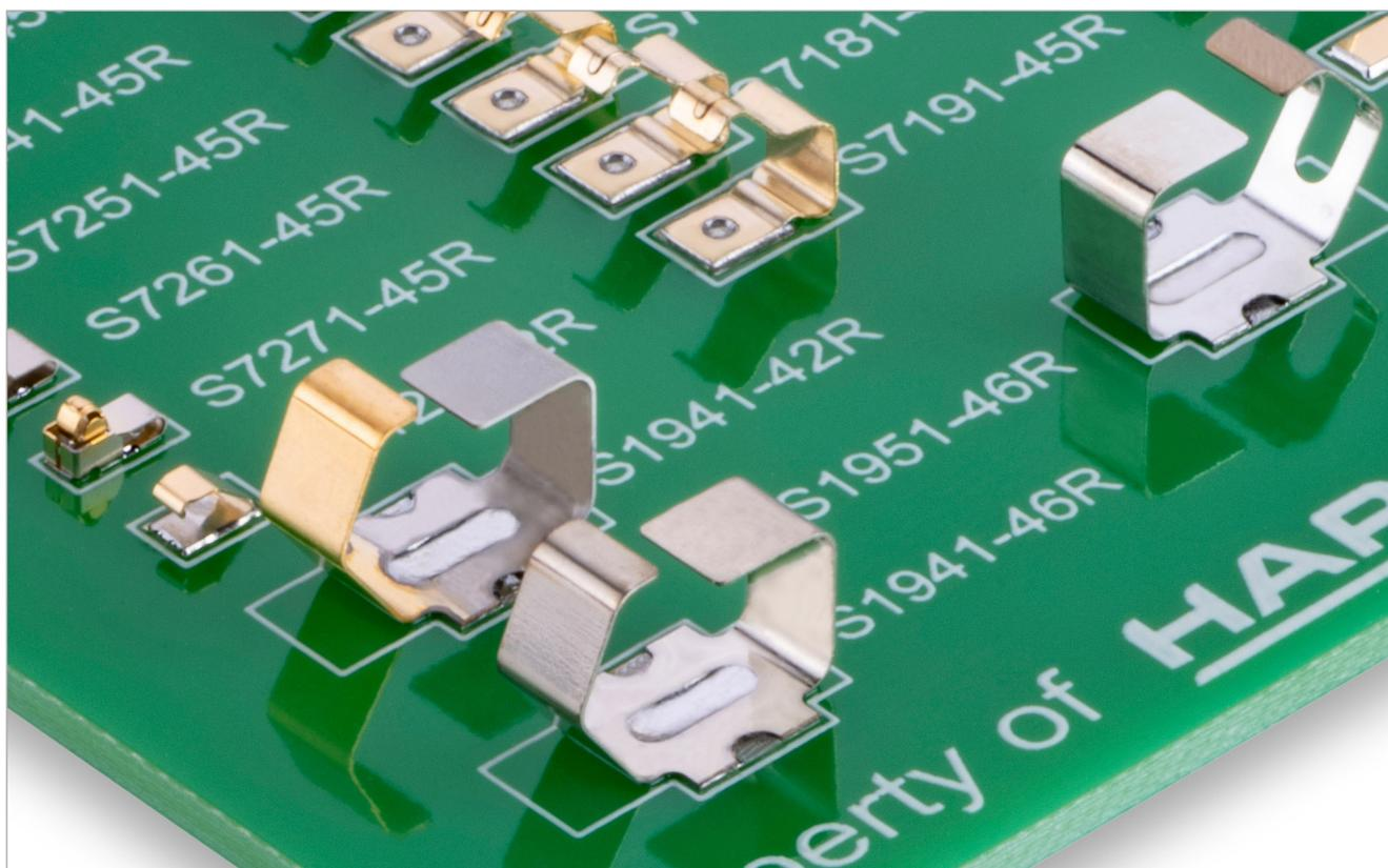
Once your electronic system is shielded from external EMI, and is not emitting EMI, now you will need to address what is happening at the board level. Here, there is the risk of individual components or devices within the system interfering with one another. The close proximity of analogue/mixed signal, RF and digital devices can cause noise coupling. Here the EMI produced by a component which has capacitive or inductive properties can affect the signal passing through neighbouring devices.
