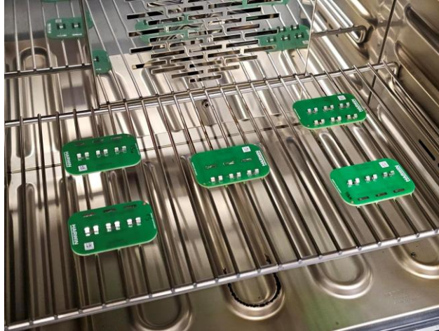
Humidity Test Setup
