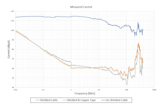
Figure 2.2.7 Measured current of the three cable assembly configuration.
