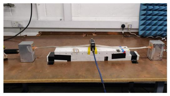
Figure 2.2.2 Test Setup: Cable assembly, braided cable with copper taping on back shells
