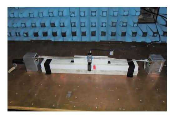
Figure 2.3.3 Test Setup: Cable assembly, braided cable with unscreened back shells
