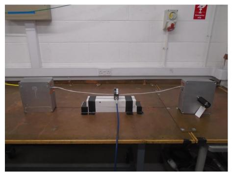
Figure 2.2.4 Test setup – 16-way, shielded cable, 1 MHz to 400 MHz
