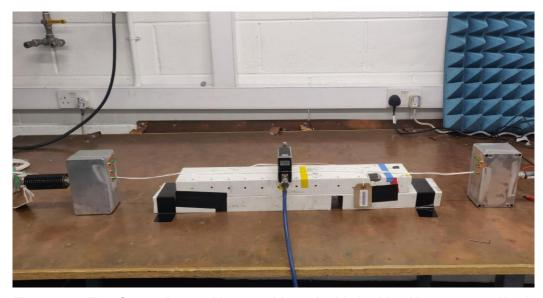
Figure 2.1.1 Test Setup: Base cable assembly, no braided cable with no screened back shells
