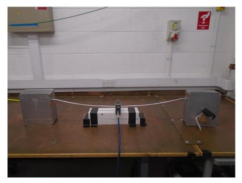
Figure 2.2.1 Test setup - 16-way, unshielded cable, 10 kHz to 1 MHz
