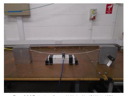
Figure 2.2.3 Test setup – 6-way, shielded cable, 10 kHz to 1 MHz
