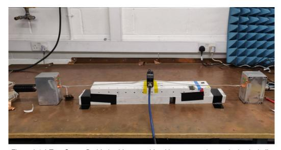
Figure 2.1.2 Test Setup: Braided cable assembly with copper taping on the back shells
