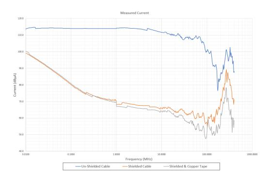
Figure 2.3.7 Measured current of the three cable assembly configuration.
