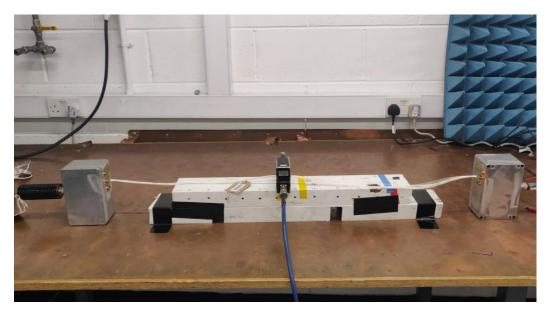
Figure 2.2.1 Test Setup: Base cable assembly, no braided cable with no screened back shells
