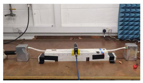
Figure 2.3.1 Test Setup: Base cable assembly, no braided cable with no screened back shells
