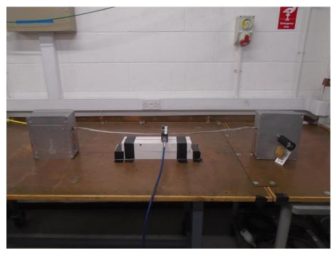
Figure 2.1.4 Test setup – 6-way, shielded cable, 1 MHz to 400 MHz
