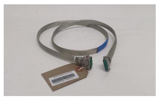
Figure 1.3.2 Equipment Under Test: Braided cable with back shells - 16-way cable assembly
