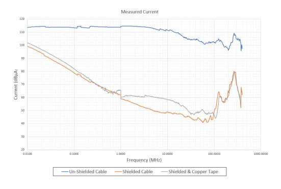
Figure 2.1.7 Measured current of the three-cable assembly configuration.
