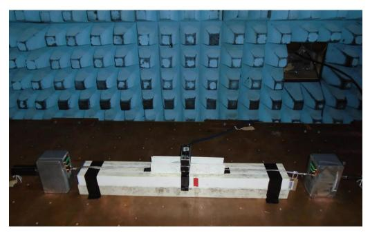
Figure 2.1.3 Test Setup: Braided cable assembly with unscreened back shells
