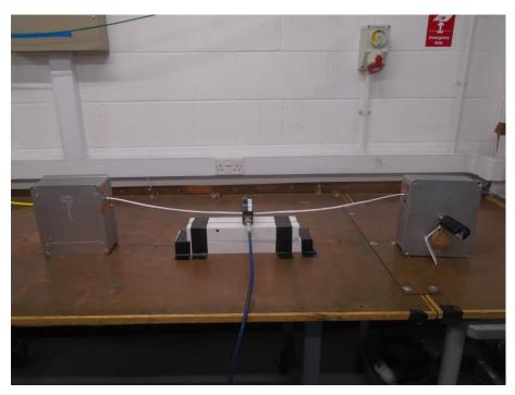
Figure 2.2.2 Test setup – 16-way, unshielded cable, 1 MHz to 400 MHz
