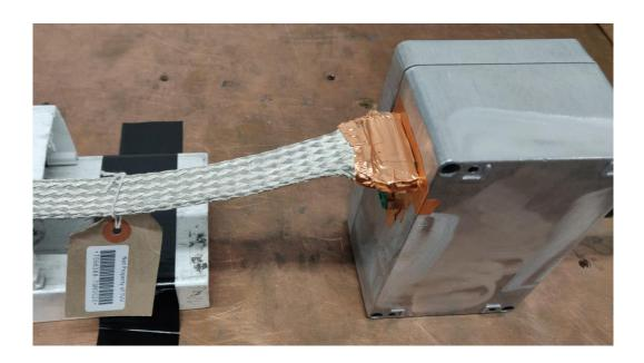
Figure 2.3.4 Copper Screening on the Back shells: 50-way cable assembly
