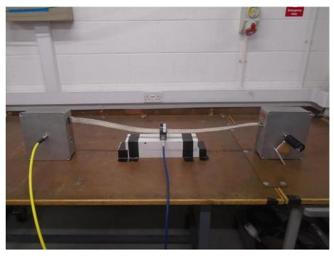
Figure 2.3.4 Test setup - 50-way, shielded cable, 1 MHz to 400 MHz
