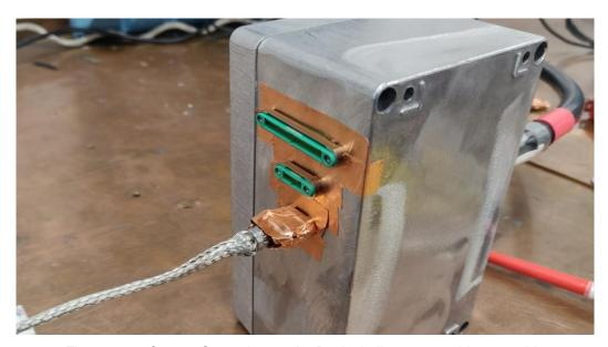
Figure 2.1.4 Copper Screening on the Back shells: 6-way cable assembly
