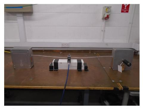
Figure 2.1.1 Test setup – 6-way, unshielded cable, 10 kHz to 1 MHz
