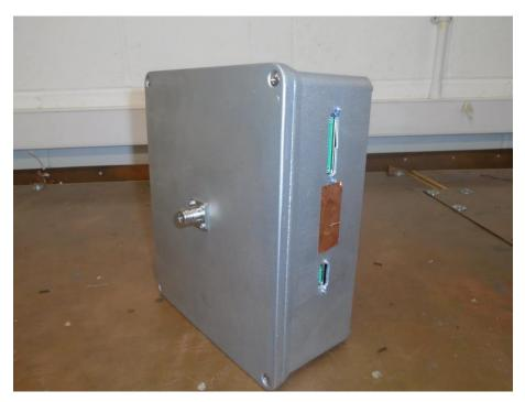
Figure 1.3.8 Interface box: side with the 50 and 6 way connectors.
