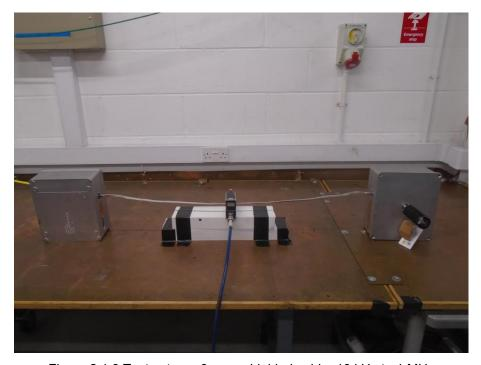
Figure 2.1.3 Test setup – 6-way, shielded cable, 10 kHz to 1 MHz
