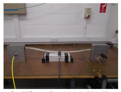
Figure 2.3.3 Test setup – 50-way, shielded cable, 10 kHz to 1 MHz
