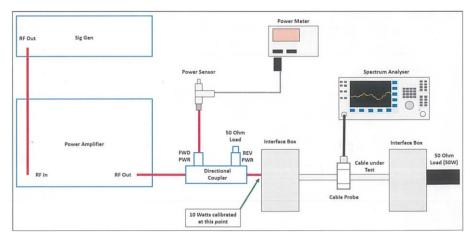
Figure 1.3.11 General test setup
