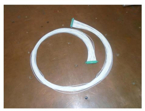
Figure 1.3.5 Equipment Under Test - 50-way cable unshielded
