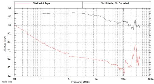
Figure 2.2.5 Shield comparison: Unscreened cable and no back shells V braid shielded cable with copper taping on the back shells
