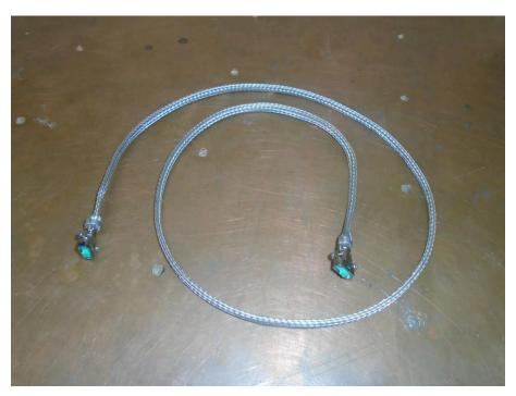
Figure 1.3.2 Equipment Under Test - 6-way cable shielded
