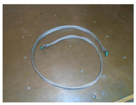
Figure 1.3.4 Equipment Under Test - 16-way cable shielded
