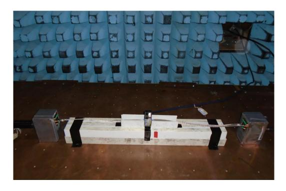
Figure 2.2.3 Test Setup: Cable assembly, braided cable with unscreened back shells
