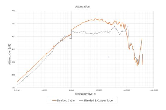
Figure 2.1.8 Attenuation achieved: Braid shielded cable with screened back shells V Shielded Cable with unscreened back shells.
