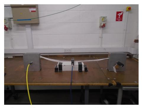
Figure 2.3.1 Test setup – 50-way, unshielded cable, 10 kHz to 1 MHz
