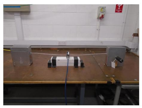
Figure 2.1.2 Test setup – 6-way, unshielded cable, 1 MHz to 400 MHz
