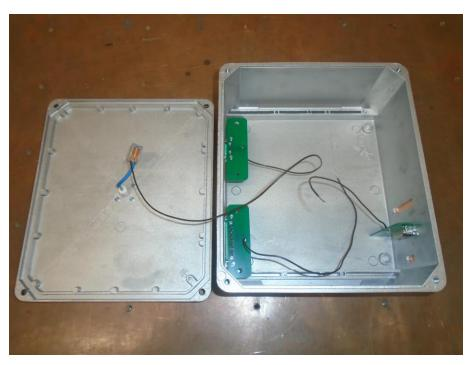
Figure 1.3.7 Interface box used to test the connectors.
