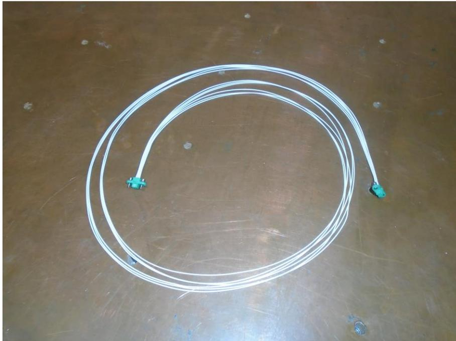
Figure 1.3.1 Equipment Under Test - 6-way cable unshielded
