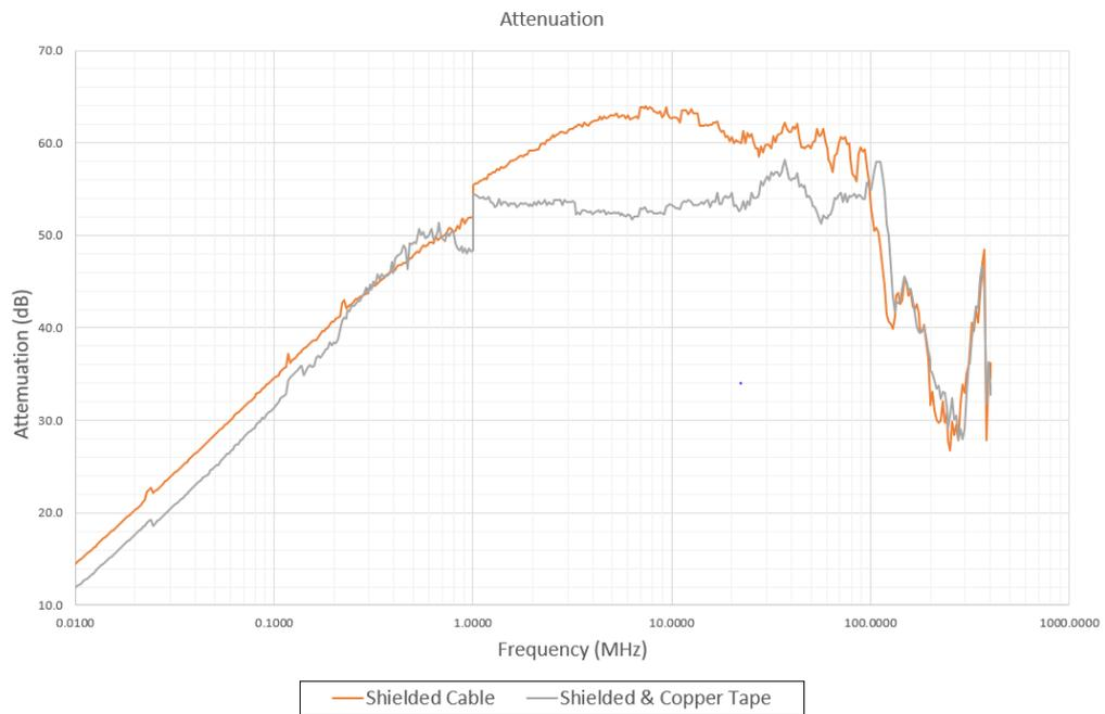
Figure 2.1.8 Attenuation achieved: Braid shielded cable with screened back shells V
