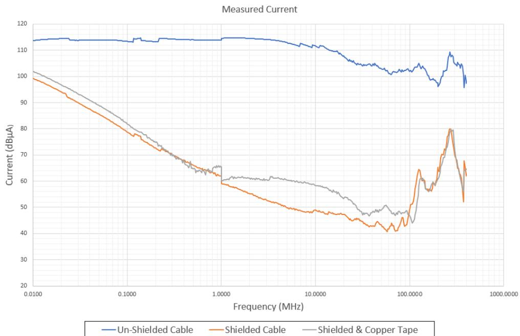
Figure 2.1.7 Measured current of the three-cable assembly configuration.
