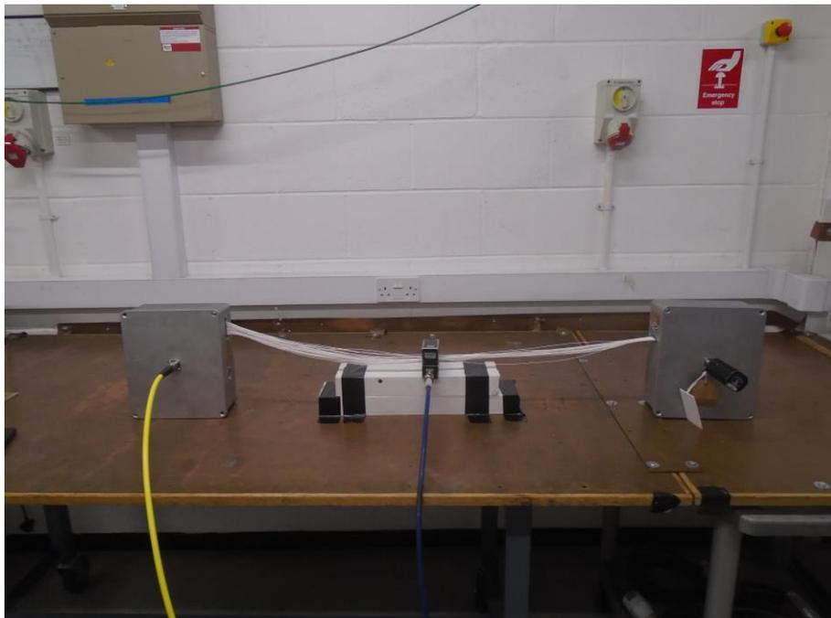
Figure 2.3.1 Test setup – 50-way, unshielded cable, 10 kHz to 1 MHz
