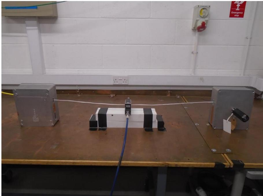
Figure 2.1.1 Test setup – 6-way, unshielded cable, 10 kHz to 1 MHz
