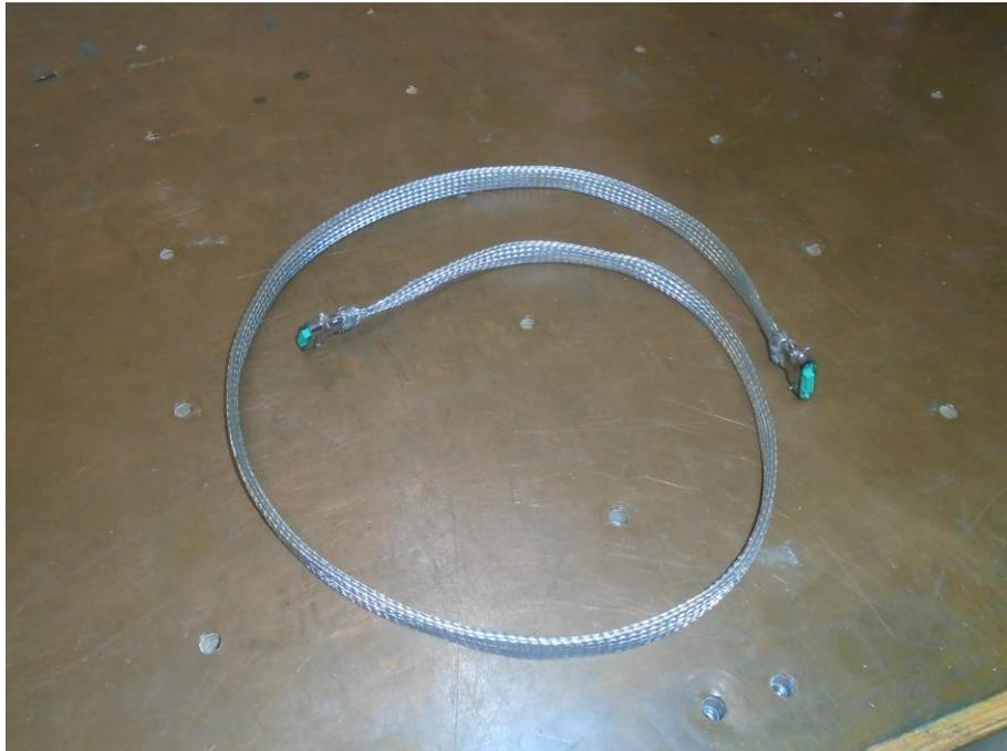
Figure 1.3.4 Equipment Under Test - 16-way cable shielded
