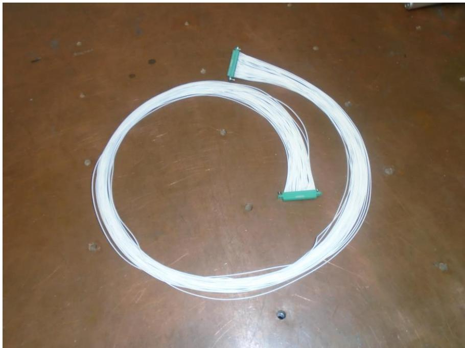
Figure 1.3.5 Equipment Under Test - 50-way cable unshielded
