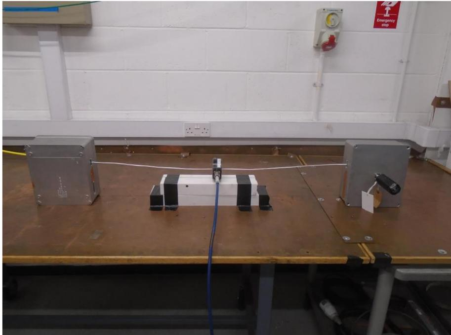
Figure 2.1.2 Test setup – 6-way, unshielded cable, 1 MHz to 400 MHz
