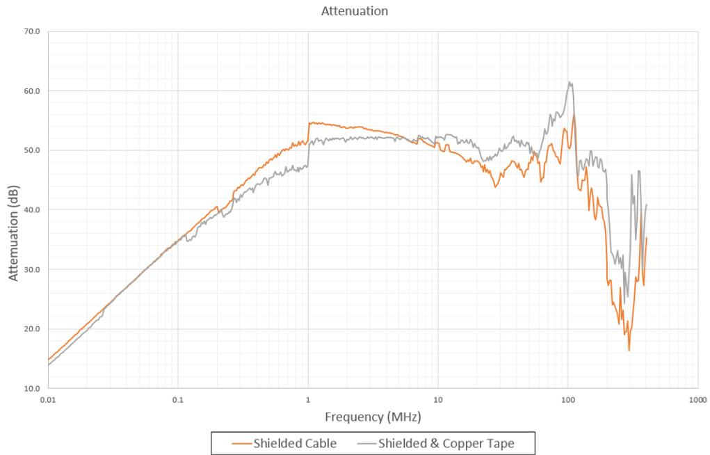
Figure 2.2.8 Attenuation achieved: Braid shielded cable with screened back shells V
