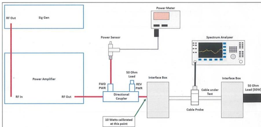
Figure 1.3.11 General test setup
