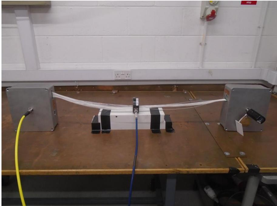
Figure 2.3.2 Test setup – 50-way, unshielded cable, 1 MHz to 400 MHz
