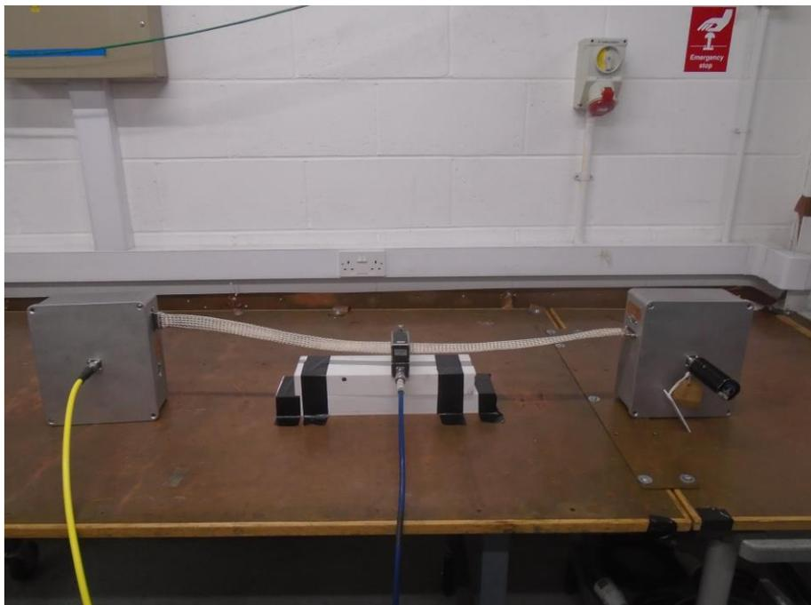
Figure 2.3.3 Test setup – 50-way, shielded cable, 10 kHz to 1 MHz
