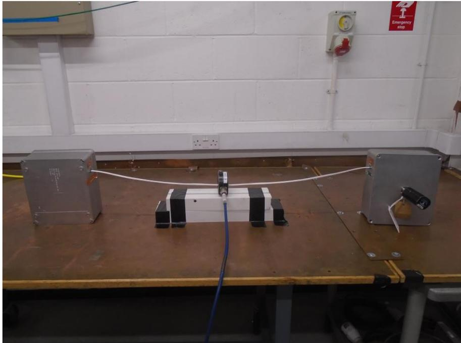
Figure 2.2.2 Test setup – 16-way, unshielded cable, 1 MHz to 400 MHz
