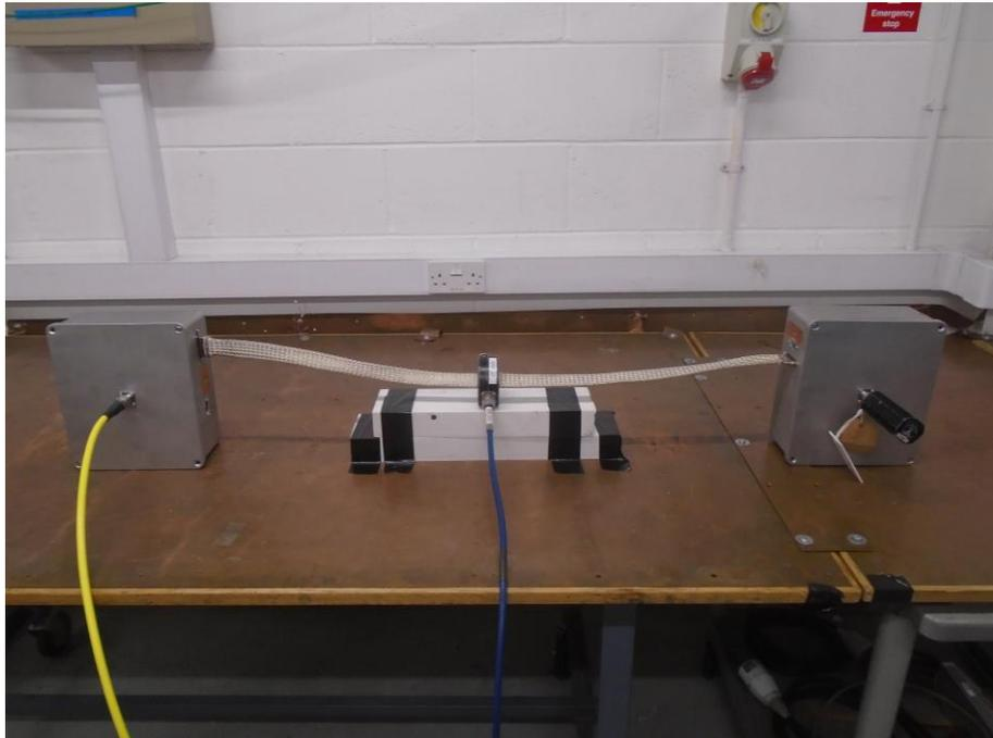
Figure 2.3.4 Test setup – 50-way, shielded cable, 1 MHz to 400 MHz
