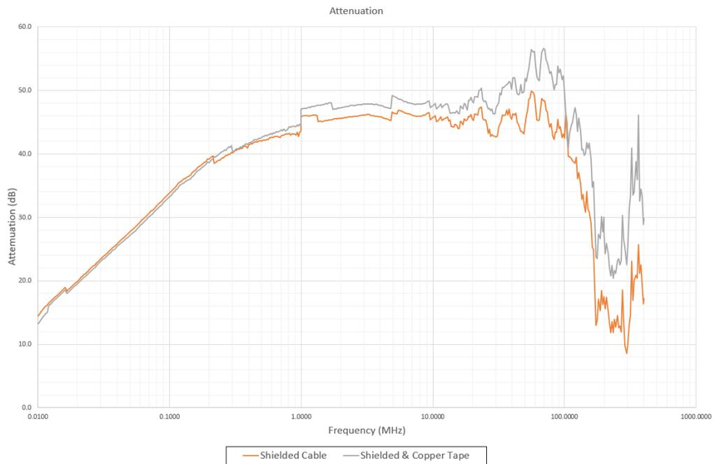
Figure 2.3.8 Attenuation achieved: Braid shielded cable with screened back shells V
