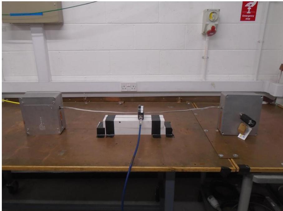
Figure 2.1.4 Test setup – 6-way, shielded cable, 1 MHz to 400 MHz
