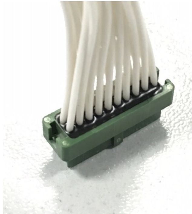
Figure 3- G125-FC12005L0-0300F after 100 hours at +150°C.
