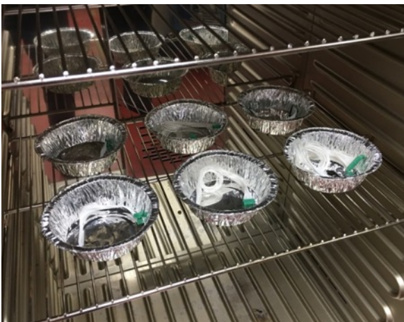
Figure 1- Arrangement of samples within the Industrial Oven.
