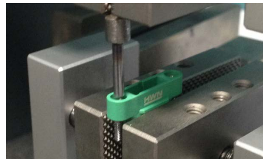
Figure 2: Testing set up with push out pin locating into the male connector.
