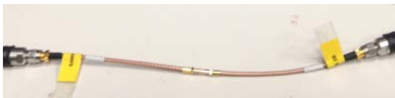
Figure 2 – Sample 2 of the cable containing the mated M80-307 and M80-317 coax contact combination
