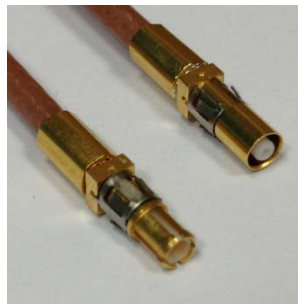
Figure 1 – The device under test, M80-307 and M80-317 coax contacts on sample 2 of the cable assembly manufactured for the test
