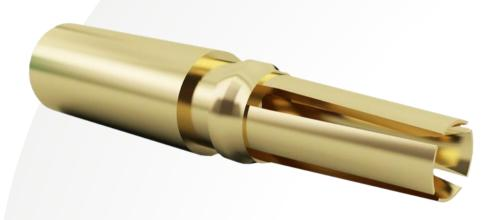
A 4-fingered Beryllium Copper female contact gives superb performance, for both electrical and mechanical specifications. These contacts are precision-turned on state-of-the art equipment at our UK headquarters, and plated with a gold finish to resist multiple insertions.
