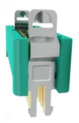
To assist with mechanical strain relief, the hold-down features have been incorporated as part of the location pegs, resulting in barbs which latch through the PCB. These barbs are designed to give retention on standard PCB thicknesses of 1.6mm and 2.4mm and are available as an option on all male PCB connectors.
