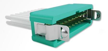
By reversing the Datamate latch design, we achieved a design improvement - it is not possible to overstress these Gecko latches during normal use. Latches are pushed in to dis-engage the mating female, instead of pulled out. This means they cannot be over-bent, as the male mating connector provides a stop point.
