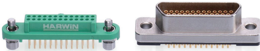
Female Micro-D (right) compared to female Gecko-SL (left)
