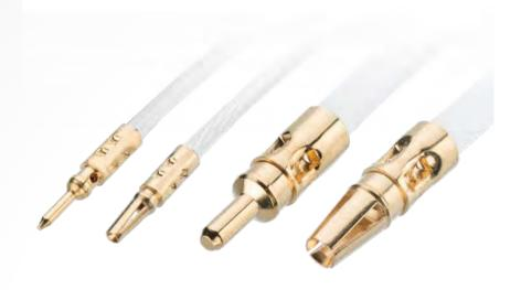
The patented single piece 4-fingered Beryllium Copper female contact gives high electrical performance and sustained mechanical durability. The crimp barrel meets IPC-A-620 specifications. It tolerates extremes of temperature, and withstands high vibration and shock. These contacts are precision-turned on state-of-the-art equipment at the UK headquarters, and plated with a gold finish to resist multiple insertions.
