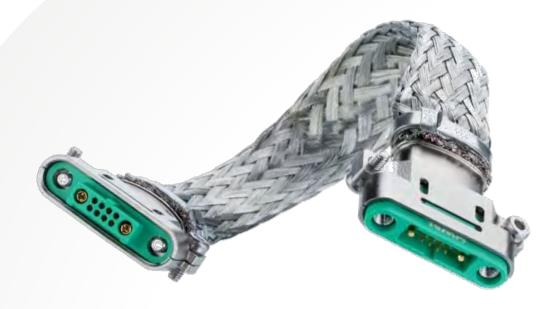
To complete the Gecko-MT range, the symmetrical connectors have been specifically designed to fit the existing 16-contact and 26-contact Gecko-SL metal backshells. This enables fully shielded cable assembly construction, with the addition of metal braiding secured around the backshells. Contact the Technical Team via our Contact page for made-to-order options.
