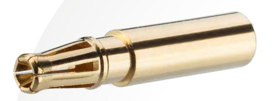
The <u>T-Contact</u> is an advanced design, based on the research around the <u>Gecko</u> connector system. By using a single piece of Beryllium Copper in a turned design, the current-carrying capacity of the contact is improved, due to additional mass of metal. Beryllium Copper is used as the base metal to ensure the spring qualities of the contact area are maintained.
