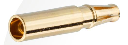
The T-Contact is available in a gold-plated finish. To maximize durability, the gold is applied at 0.76-1.00µm (30-40µ") thickness, over nickel & copper undercoats. Durability is increased from the existing 500 mating cycles to 1,000 mating cycles without degradation. This meets the more demanding standards of the military and aerospace requirements.
