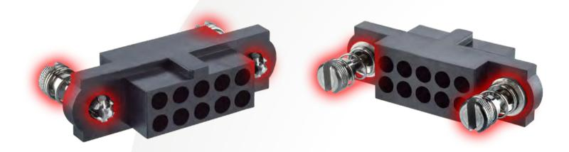
The 101Lok fixing system is a bayonet-style, <u>fast-acting method</u> of securing mated pairs. Simply mate the connectors together, then push and turn each fixing by 101-degrees (just over a quarter-turn). To disengage: push, rotate in the opposite direction and release. For a complete part number, replace the "xx" with the total number of contacts required – from 04 to 50.
