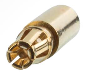
The contact design uses 6 fingers to increase the amount of contact with the mating male pin. The pattern of the 6 fingers has been likened to a Turtle shell hexagonal pattern – hence T-Contact.
