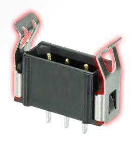
The Datamate L-Tek connectors use simple locking latches made from high strength Beryllium Copper. Mating is fast and simple – just push the two connectors together, and the latches snap into place. The connectors are then locked together and require manual deflection of the latches to separate.
