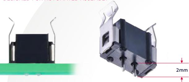
Datamate connectors typically have 3mm terminations, to give robust throughboard connection with wave soldered or hand soldered joints on the underside of the PCB.
