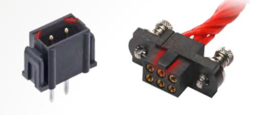
All Datamate styles feature shrouded male and female connectors, to prevent accidental damage to the miniature contacts. As the connector housings have shrouding, they can also incorporate Polarization. This prevents connectors being mated upside-down.
