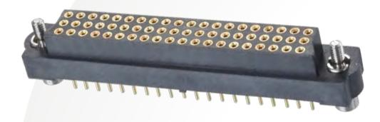
Datamate connectors are all based on a 2mm pitch system, with contact counts from 2 to 96. This compact system gives improved current rating over classic 2mm pitch pin header and socket systems, as well as meeting the high-reliability requirements with the vibration and temperature specifications.
