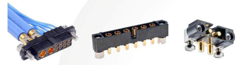
Datamate Mix-Tek uses the same outer housing design as Datamate J-Tek, with each power contact taking up the space of 4 signal contacts (giving 4mm pitch). The original power contacts are capable of up to 20A, and the latest <u>High Power</u> contacts will carry 40A each.
