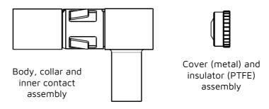
3) Push the cable into the body, as far as it will go. The cable inner conductor will be visible through the hole in the back of the coax body, and should go into the slot in the inner contact.
