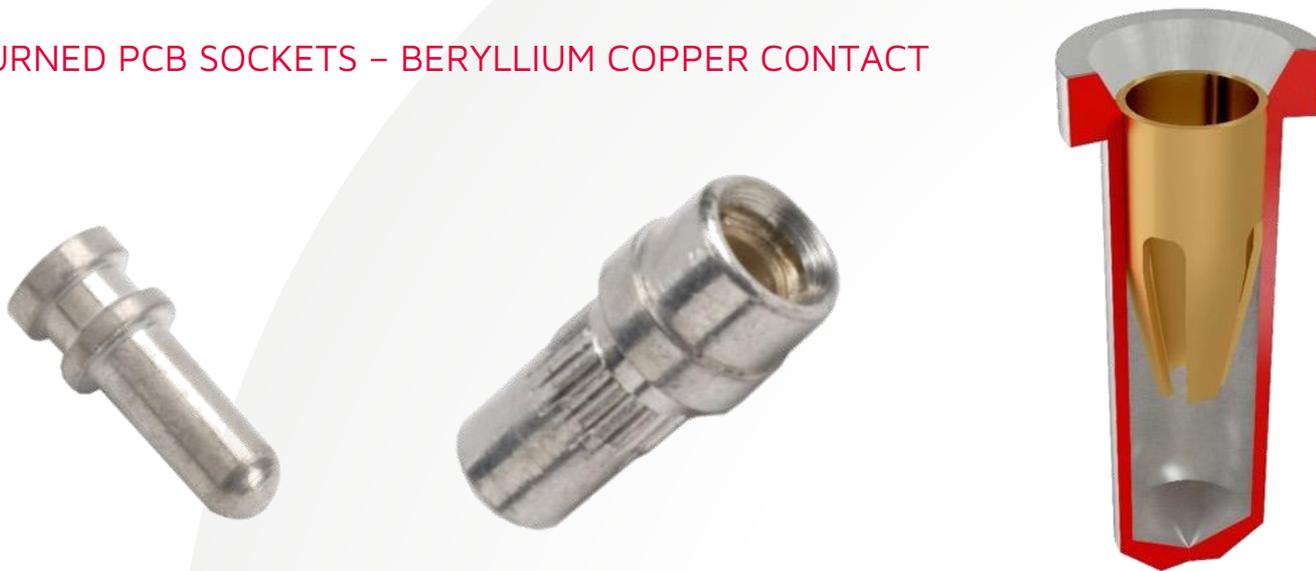
The construction of the [turned body PCB socket](#) uses the same technology as the High-Reliability connectors in the Harwin range (Datamate and M300). A Four-finger Beryllium Copper clip is mounted in a turned Brass shell. This four-finger clip design gives excellent performance under shock and vibration in all 3 axes. Current ratings are also excellent, and mating cycle durability exceeds 500 operations.
