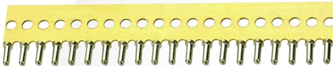
Generally, sockets are provided loose packed. However, to assist with the small size, the Ø0.5mm sockets (Sub-miniature) are also supplied on a metal comb carrier strip, for semi-automated or assembly in rows, on a pitch of 2.54mm.
