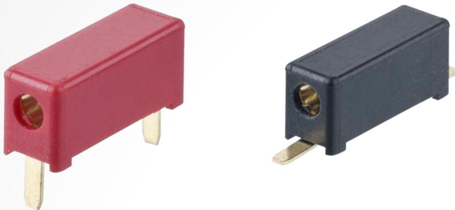
The Test Socket from Harwin is a horizontal, dual-entry socket, compatible with Ø2.03 test probes and other Ø2.00mm mating pins. It has a low profile height of 5.1mm above the PCB.
